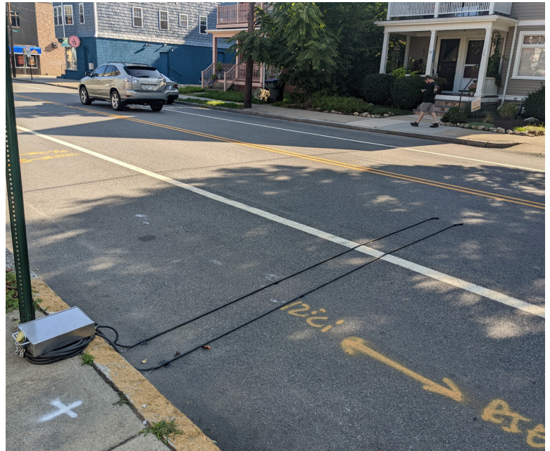
Temporary pneumatic tube counters on Hope Street
